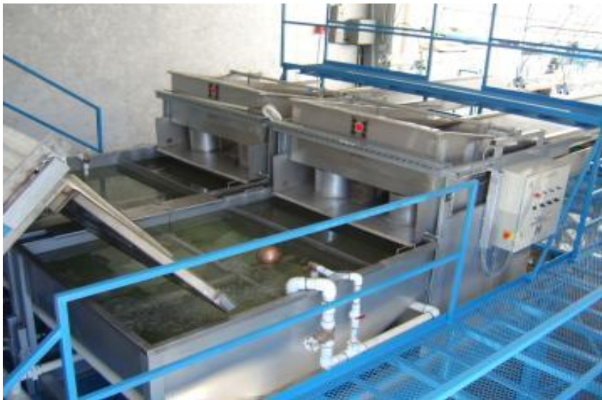
Two high capacity cluster separators in parallel = 4 tons / hour
