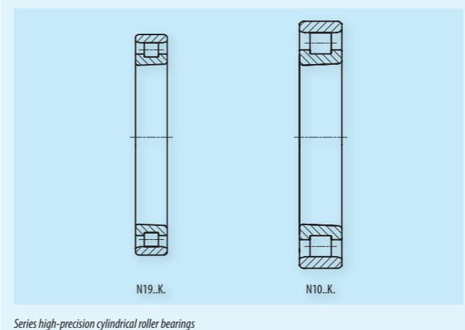
Series high-precision cylindrical roller bearings
