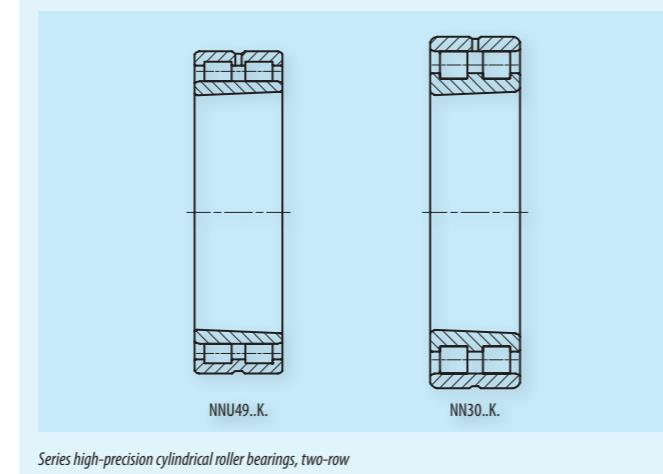
Series high-precision cylindrical roller bearings, two-row
