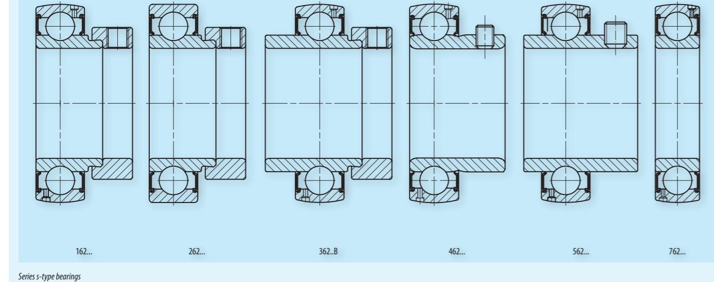
The first five series are provided each with a wide inner ring. These bearings are fixed at a shaft either by means of an eccentric ring (series 162..., 262... and 362...B) or with two threaded pins (series 462... and series 562...).
