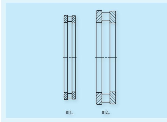
Series thrust cylindrical roller bearings, single-row
