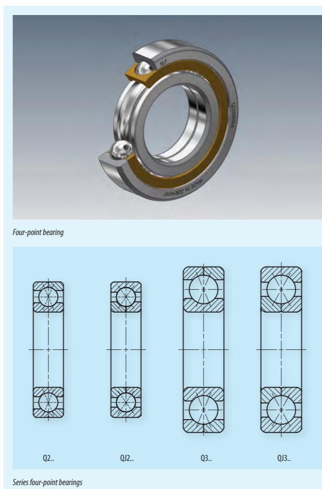
Due to the split inner resp. outer ring it is possible to place a high number of balls. Relevant ring (outer or inner ring) with ball race and relevant ring halves can be installed separately. The angular adjustment facility is very low.
