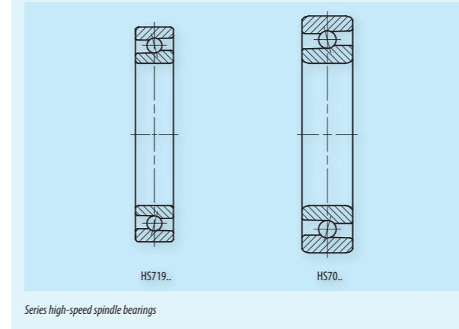
Series high-speed spindle bearings
