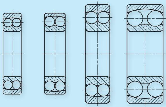
Series self-aligning ball bearings
