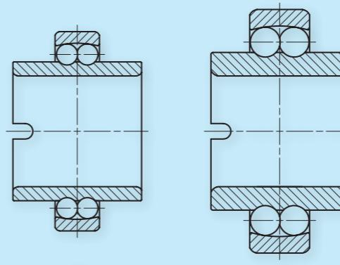
Series self-aligning ball bearings with wide inner ring
